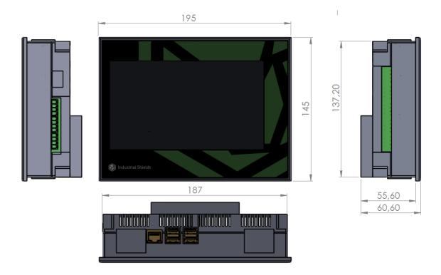
Panel Touch 7" is designed to be placed build-in an electrical box. Next it is showed the dimensions to be installed properly:
