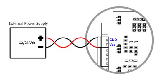
Find attached a picture regarding the position of the external power inputs:
