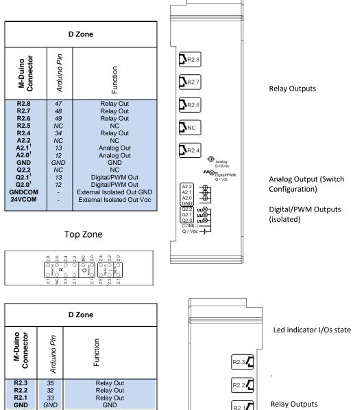
**Relay Outputs** R2.1 Analog: 0-10Vdc Digital: 5 - 24Vdc Digital: 5 - 24Vdc \* Note: use correctly configuration to use this signal. (see user guide) Analog/Digital Inputs Interrupt Inputs (isolated) Configuration Switch\* (see section 8 to select the correct configuration for
