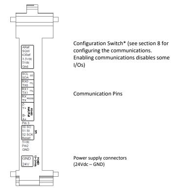
SS: Chip Select pins. These pins can act as TTL, so they can work for the Chip Select pin of any device.
