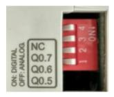
For the Relay Shield if a switch is set to ON, it can only act as Digital Output. If it is set to OFF it can only act as an Analog Output.
