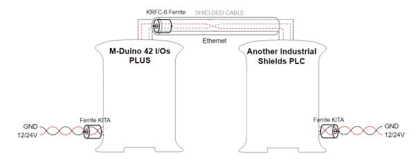
For an Ethernet communication between Industrial Shields equipment a **SFTP CAT-6 Ethernet crossover cable** must be used.
