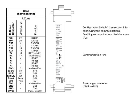
SS: Chip Select pins. These pins can act as TTL, so they can work for the Chip Select pin of any device.
