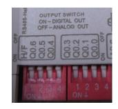
**RIGHT ZONE.** The right zone configures the outputs. If the switch is set to "ON" the Q0.X will have the behaviour of a digital output. If it is set to "OFF" it will be analog. There is also a switch for switching between Half and Full Duplex. It is "ON" for Half Duplex and "OFF" for Full Duplex.
