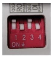
NOTE: Although in the TOP ZONE serigraphy it is shown Q0.9 & Q0.8 pins, in the reality they are I0.3 IO.2 pins respectively. Additionally although the serigraphy only is expressed for the RS485 it is also the same for the RS232. So if it is desired to enable any of the Hardware Serial connection this is the function of these switches. See chapter 8 for more information
