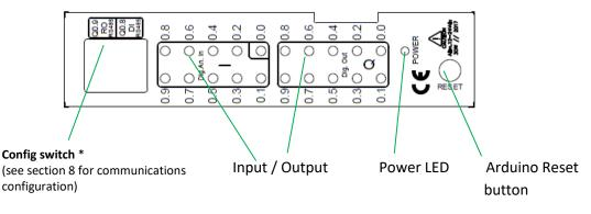
NOTE: Although in the TOP ZONE serigraphy it is shown Q0.9 & Q0.8 pins, in the reality they are I0.3 IO.2 pins respectively. Additionally although the serigraphy only is expressed for the RS485 it is also the same for the RS232. So if it is desired to enable any of the Hardware Serial connection this is the function of these switches. See chapter 8 for more information
