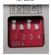
NOTE: Although in the TOP ZONE serigraphy it is shown Q0.9 & Q0.8 pins, in the reality they are I0.3 I0.2 pins respectively. Additionally although the serigraphy only is expressed for the RS485 it is also the same for the RS232. So if it is desired to enable any of the Hardware Serial connection this is the function of these switches. See chapter 8 for more information
