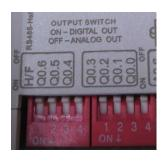
**RIGHT ZONE.** The right zone configures the outputs. If the switch is set to "ON" the Q0.X will have the behaviour of a digital output. If it is set to "OFF" it will be analog. There is also a switch for switching between Half and Full Duplex. It is "ON" for Half Duplex and "OFF" for Full Duplex.
