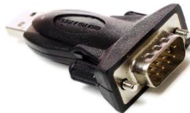
Figure 2: USB to RS232 converter
