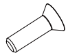
35 Hexagon socket countersunk head screw (black) M4X14 x 1 内六角沉头螺钉(黑)M4X14
