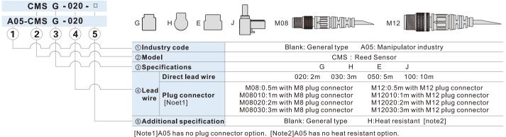
[Note1]A05 has no plug connector option. [Note2]A05 has no heat resistant option. Add:The sockets of M08 and M12 need additional order. Please check on page 585.
