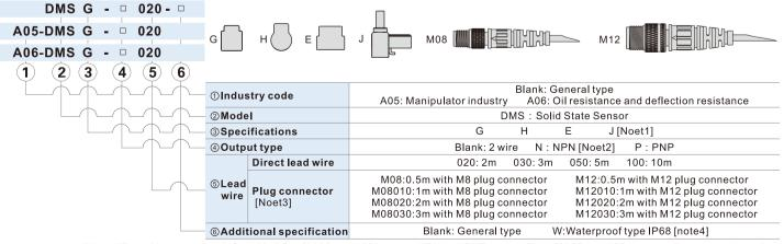
[Note1]Type J is not available for A06. [Note2]A05 and A06 have no NPN and PNP option. [Note3]A05 and A06 have no plug connector option. [Note4]A05, J type and M08, M12 don't have a-w Waterproof option. Standard A06 model already has a waterproof function. Add: The sockets of M08 and M12 need additional order. Please check on page 585.
