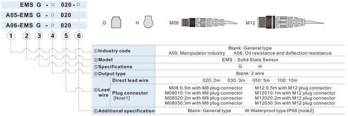
[Note1]A05 and A06 have no plug connector option. [Note2]A05 and A06 don't have a-w Waterproof option. Standard A06 model has a waterproof function. Add:The sockets of M08 and M12 need additional order. Please check on page 585.
