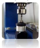
As it was mentioned at the beginning — to set the material base we are going to use the carbide roller, filed precisely on half of diameter. If we use tool length measurement, then enter the tool num-
