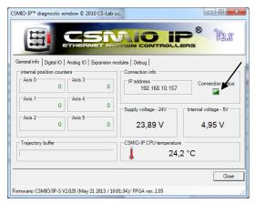
You will see CSMIO/IP diagnostic window. If the "Connection status" light is green it means that the firmware was installed correctly and communication between Mach3 software CSMIO/IP controller is also correct.
