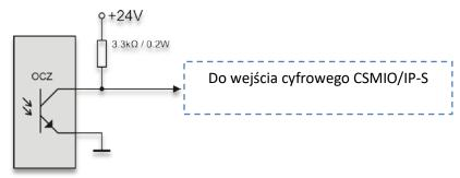
As it is shown - pull-up resistor is enough. However sometimes we do not have "open collector" —type output available, then the only way for homing on index is to add external, simply electronic system:
