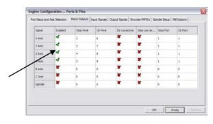
At the beginning, you should activate support of the axes you are going to use. Select the menu position "Config" Ports and Pins" and next "Motor Outputs" tab.
