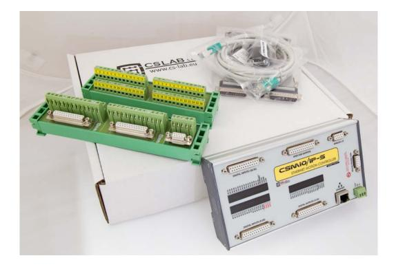
The CSMIO/IP-S set includes terminal block adapters for easier wires connection in a control cabinet. More content details below:
