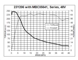
something about 200 rpm - the torque is almost the same (pictures below), but with increasing revs the torque, actually the power on the motor shaft), decreases drastically. It decreases to such low value that sometimes happens that at 1000 rpm. the motor has no power to work itself, not saying about propelling the machine.
