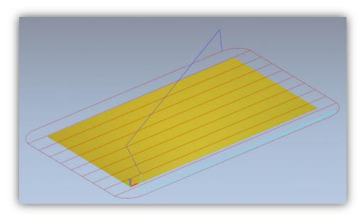
Now we record the trajectory, go to the Toolpaths tab and click the 📽 icon. In the record window, select so-called postprocessor, to define output data format suitable for our control system. In ArtCam we recommend "G-Code Arcs (mm) (\*.tap)". It is basic G-Code format suitable for Mach3 software. When you select the format pres "Save" and save our trajectory as e.g. "planning.tap".
