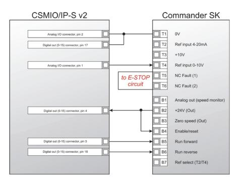
In the example above, you can see the simplest connection of an inverter to operate spindles in an engraving plotter.
