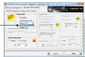
Again, during the startup the diagnostic window may be helpful. In the "Analog IO" tab, you can preview current voltages on analog inputs and outputs. When we configure the spindle, then in a MDI tab you can enter e.g. M3 (enter), S2000 (enter). It should cause spindle activation (right revs) and setting the revs on: 2000 rpm. In the diagnostic window, you can see digital outputs and voltage on analog output activated.
