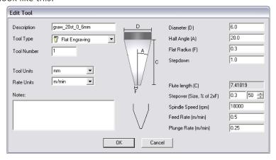
You should note that, in ArtCam software a handle size is given as diameter, and a dimension of tip of the tool (F) is as radius. Speed values in here are quite low but it is only example, and not "high performance ride", which
