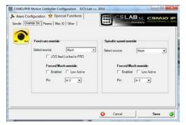
In "Override sources" tab you can set whether the speed adjustment should be done through Mach3 screen, analog inputs or additional MPG encoder axes, etc.
