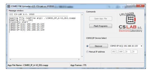
If you run the update application from installer file it means that correct file with the firmware was already loaded and "Open App. File" button is not active. If there is only one CSMIO/IP controller in network - the application asks to start the update automatically. If there are more controllers then you should chose one IP address from a list to update the controller you want and click "Flash Programm".
