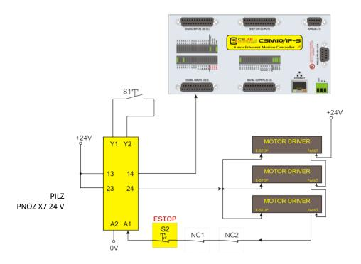
Above you can see an example of E-Stop signal connection to the CSMIO/IP-S controller and to the axis drives, using Pilz company safety relay (PNOZ X7 24V symbol). S1 is a reset button (switching on the safety relay), S2 is the emergency stop. The safety relay is an option, it's not required.
