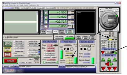
Now use arrow keys or keys on a machine desktop, reach left edge of the material. Z-axis is a little below the material level.
