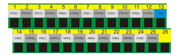
By default, axes are assigned to following channels STEP/DIR: X→[0] / Y→[1] / etc.
