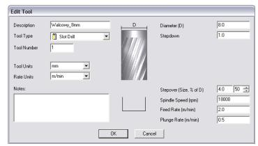
ment last longer. Feed Rate is a feed on XY surface, and Plunge Rate means speed with which the tool will get into the material. Tool Type is a tool shape type. Here the drawing, displayed after shape type selection, is helpful.
