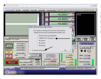
Select motion controller type – "CSMIO\_IP/P" and fill in the check box: "Don't ask me again", so Mach3 in this configuration profile will always use CSMIO/IP-S controller. Confirm your selection with "OK".
