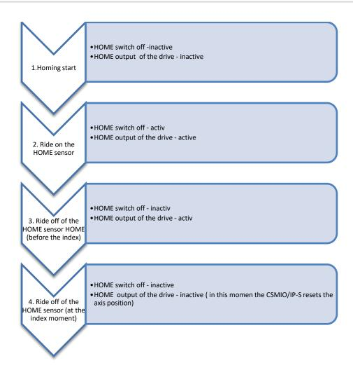
As shown on the diagram above, the drive should extend the active state on the HOME output until it step on the encoder index. During the tests with simDrive the achieved homing accuracy at 2000mm/min speed and encoder's 10000imp/rev - ranged +/-1 imp. of the encoder.
