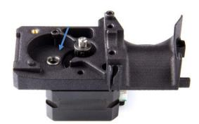
• Insert a ball bearing. Ensure it is fully pressed down into the slot.
