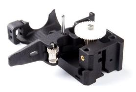
• Install the hinge to the extruder rear using the 3x32mm shaft.
