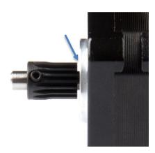
Leave a 1-1,5 mm gap between the gear and the motor and tighten it using your 1,5mm Allen key.
