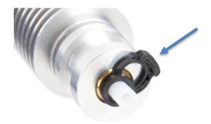
Use a knife or razor to chamfer the inside of the tube for better filament guidance.
