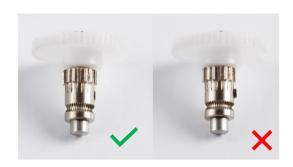
Important: If the setscrew is not properly aligned with the flat surface it will stick out and start grinding on the secondary drive gear when you start printing!
