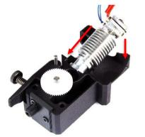
Install the HotEnd into the extruder rear, angled as shown in the photo. And push it in place.
