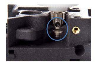
• Insert the M3x2 setscrew and tighten it with your 1,5 Allen key.
