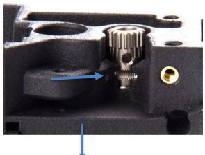
Press the primary drive gear down until the groves align with the filament path.
