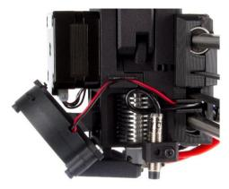
The position of the P.I.N.D.A probe depends on your version of the printer. MK2/s users place the probe to right (Closer to the Xaxis) MK2.5 and MK3 users place the probe to the left (furthest away from the X-axis).
