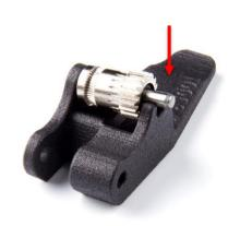
Align the gear with the hinge as shown in the photo and press the shaft down until you hear the click.
